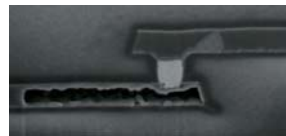
Extrusion to a bond wire causing a short circuit.
