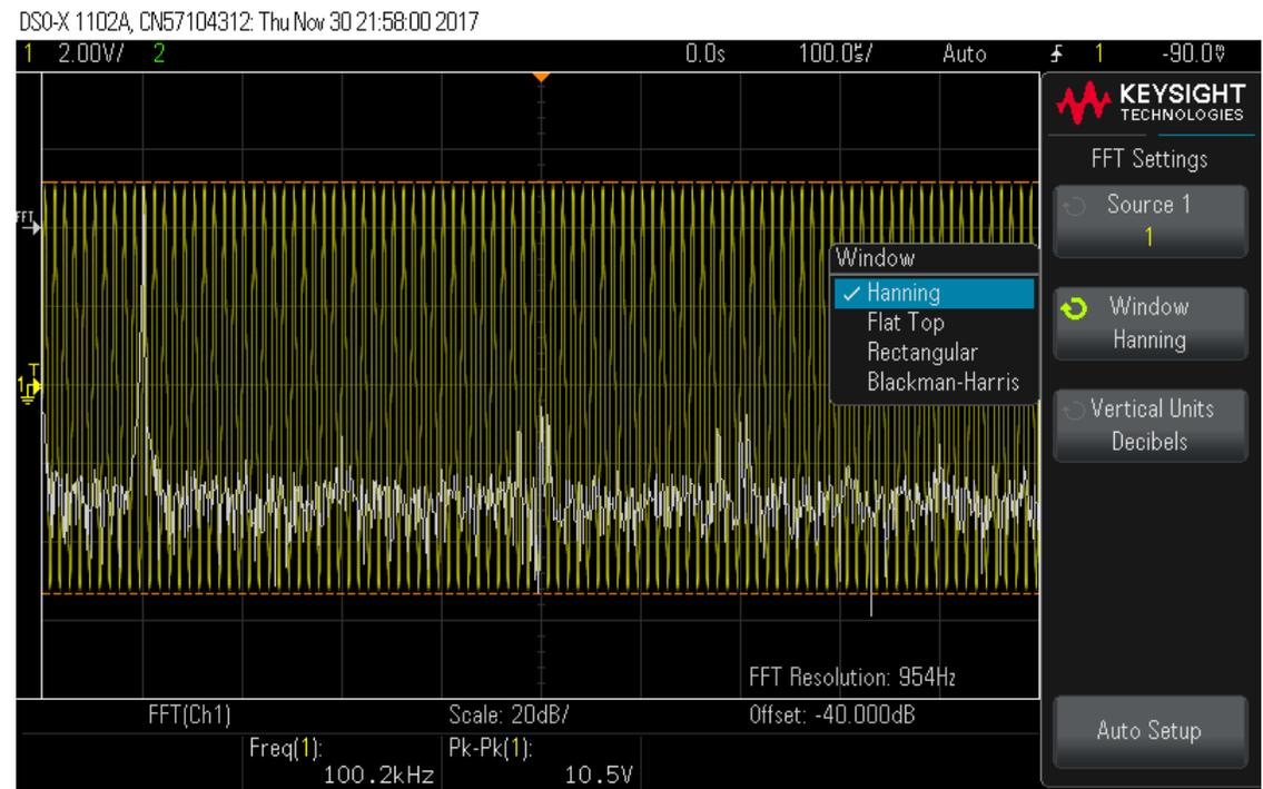
Signal sinusoïdal,  $f_0 = 100 \text{ kHz}$ ,  $F_e = 2 \text{ GHz}$ ,  $NT_e = 100T_0$
