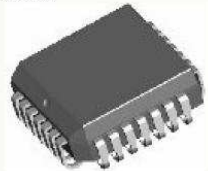
Plastic Lead Chip Carrier (PLCC) here: PLCC28
